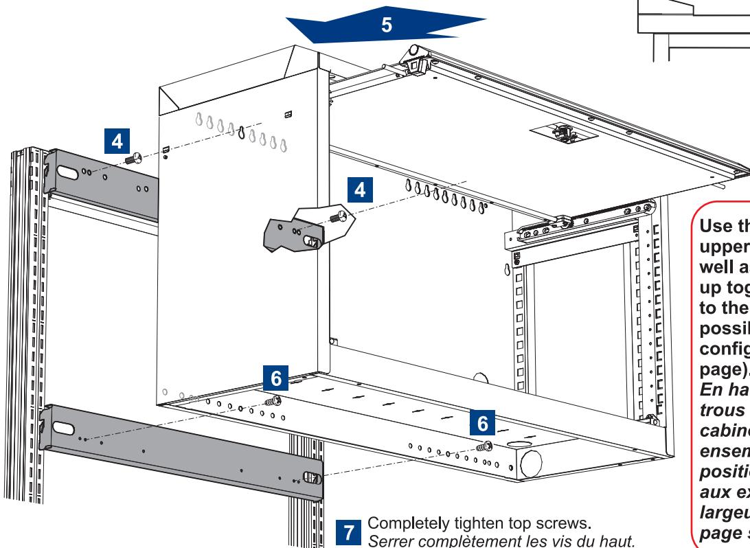
**Use the holes on both the upper and lower bracket, as well as on the cabinet that line up together and are as close to the edge of the cabinet as possible (as per the configurations on the next page).**
