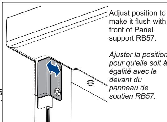
Adjust position to make it flush with front of Panel support RB57.
